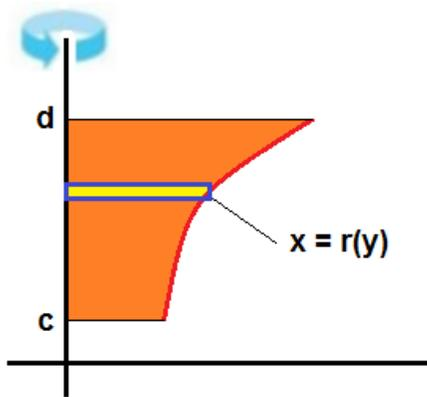
In this case, we accumulate rectangles from  $c$  to  $d$ ; these rectangles generate “stacked discs” of radius  $r(y)$ . The comparable formula is
